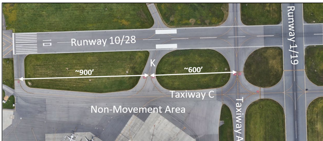
Figure 4-11 – Non-Standard Runway to Taxiway Separation
