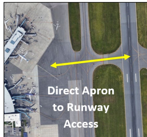
Figure 4-10 – Direct Apron-to-Runway Access
